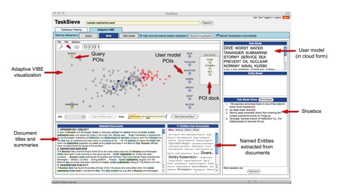
Figure 3: Prototype System User Interface - Visual TaskSieve (TaskSieve plus Adaptive VIBE)
