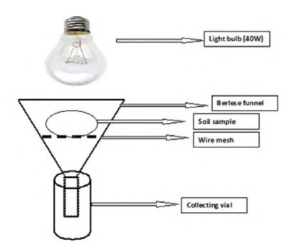
FIGURE 1: Diagrammatic view of Berlese funnel extraction apparatus
